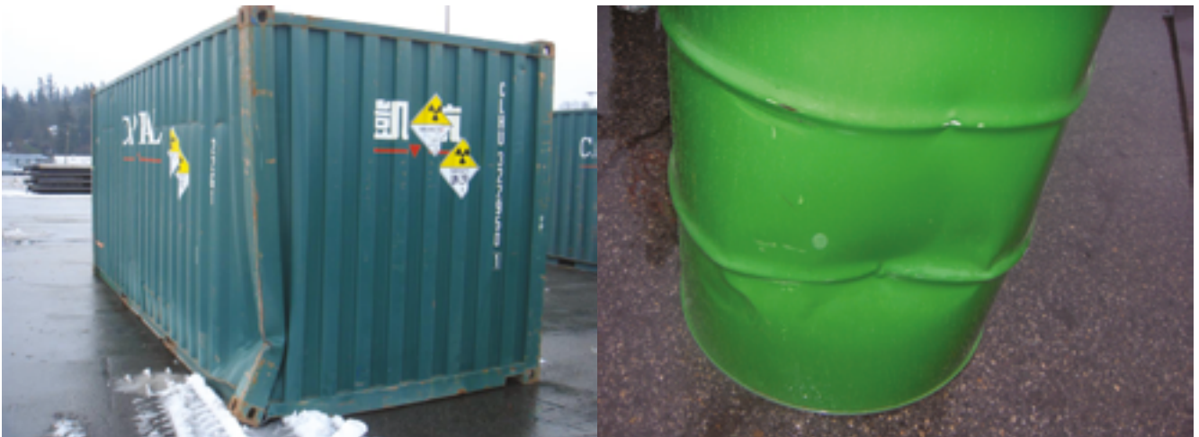
Figure 9.1: Damage to UOC shipping and packaging containers
