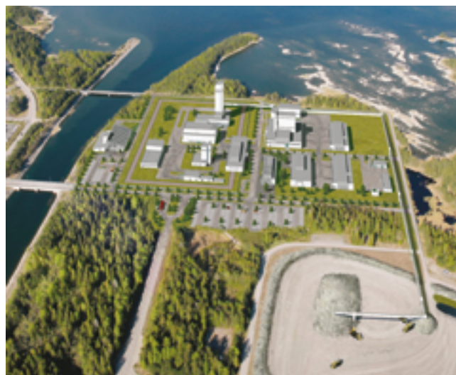
Figure I.14: Aerial photo overlay with artist's impression of the site for Sweden's used fuel disposal facility. The surface facilities will be clustered near the cooling water channel to the nearby nuclear power plant
