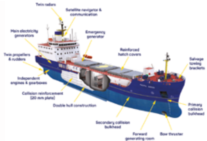
Figure 9.3: A schematic of an INF 3-rated ship, purpose-built to transport used nuclear fuel packages
