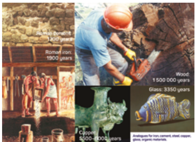
Figure I.9: Examples of materials preserved over long periods in conditions similar to a GDF
