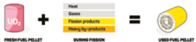
Figure 5.7: The chemical make-up of used fuel
